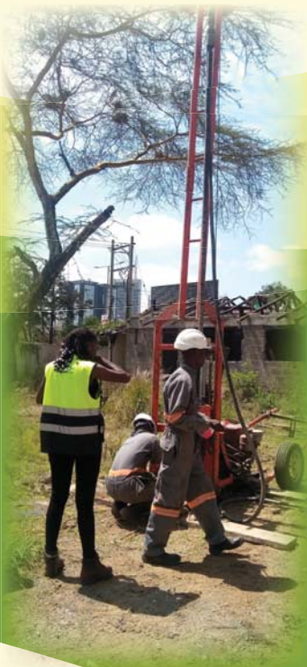
Geotechnical surveyors working on the Upperhill medical center construction site to advise AIH whether it would be possible to dig the foundation to create four basement parking.
